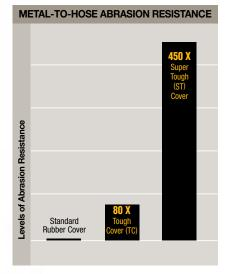
Results from the ISO 6945 metal-to-hose abrasion test show that Tough Cover and Super Tough cover hoses offer significantly greater abrasion resistance than standard rubber cover hose.
