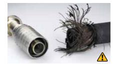
To mix and match components is to increase the risk of hose failure – a dangerous situation regardless of setting or application.
