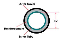
The hose size is determined by the inside diameter which can be measured or found on the layline. Parker uses a system of measurement called Dash Numbers to indicate hose and fitting size. The dash number, or dash size, is the measure of a hose's Inner Diameter (I.D.) in sixteenths of an inch. (The exception to this is SAE 100R5 hose. See the chart below for complete details.)
