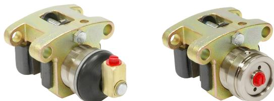
The MICO 515 **Spring Apply, Hydraulic Release** design uses a stack of Belleville springs to apply the brake and hydraulic pressure from a source such as a master cylinder to release the brakes. This design can be used with a rotor 5/16 to 1/2 inch thick having a diameter of 6 inch or larger.
