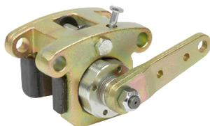
The MICO 515 **Hydraulic Apply** design uses a modulated hydraulic pressure source, such as a master cylinder, to control brake torque. These brakes use a 1 1/2 inch diameter actuation piston. They are
