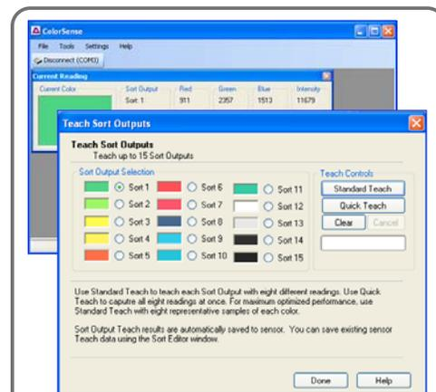
**Use ColorSense to select options, adjust parameters, and optimize the CS24D to your specific application.**
