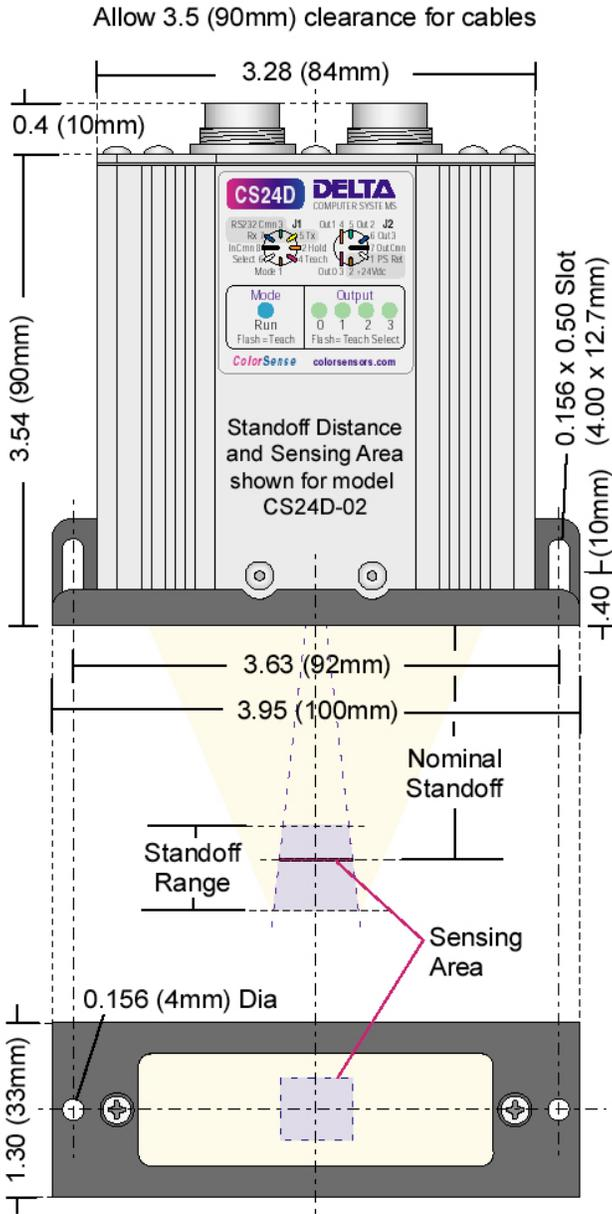
The CS24D is available in several models with a variety of sensing areas and standoff ranges. Standoff ranges include 0.63 to 1.00" (16 to 25mm) and 1.50 to 2.13" (38 to 54mm) shown above.
